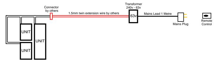
The standard items supplied with the units is 300mm of 1.5mm(2) wiring attached to the sealed unit, 1x240v - 63v transformer, 1x mains plug and lead (1 metre).
